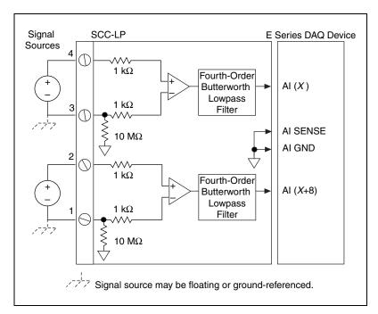
Figure 1. SCC-LPXX Signal Connections
